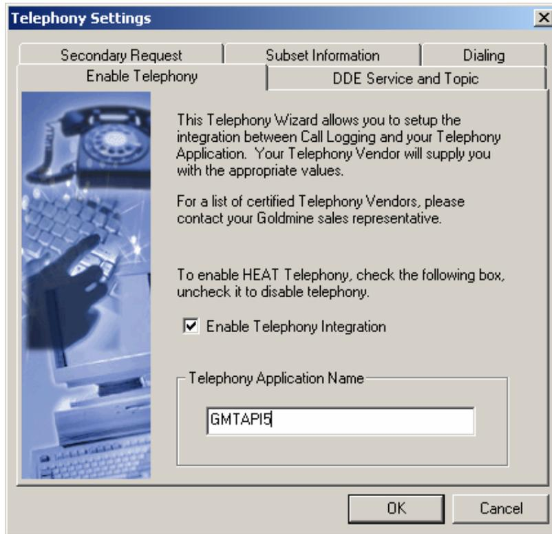
The Telephony setup allows the personalizing of several settings. On the **DDE Service and Topic** tab it is possible to name the DDE Service and Topic names as well as define the DDE Service and Topic names used by Call Logging to call the Telephony software.
